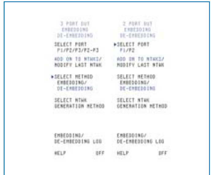
Figure 7. The initial menus for two and three port DUTs are shown here. The choices to be made are basically the same as for four port DUTs except the configuration is strictly single-ended for two port devices and only ports 2 and 3 of a 3 port device can be considered balanced.
